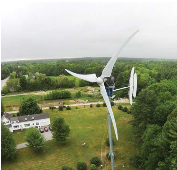
A small wind electric system may make sense if you live on at least one acre of land and have an ample wind resource.
