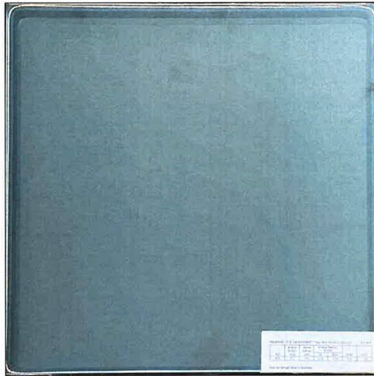
1" OVERALL CLEAR – 5,000 SQ.FT : 1/4" SOLARBRONZE TEMP – LOW-E: GUARDIAN SUNGUARD® SNX 62/27 OR EQUAL ON #2 1/2" SPACE ARGON FILLED & 1/4" CLEAR TEMP
