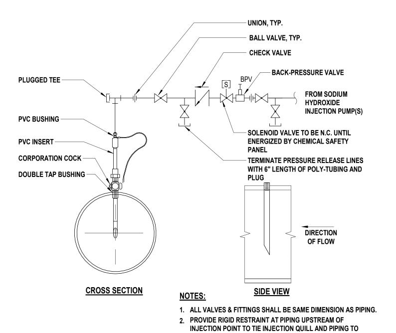
**Caustic Injection Tap Detail**SCALE:NTS
